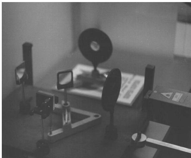
Figure 2. It is an actual photo of the lab and the modified set-up of the interferometric device (Twyman-Green interferometer).
