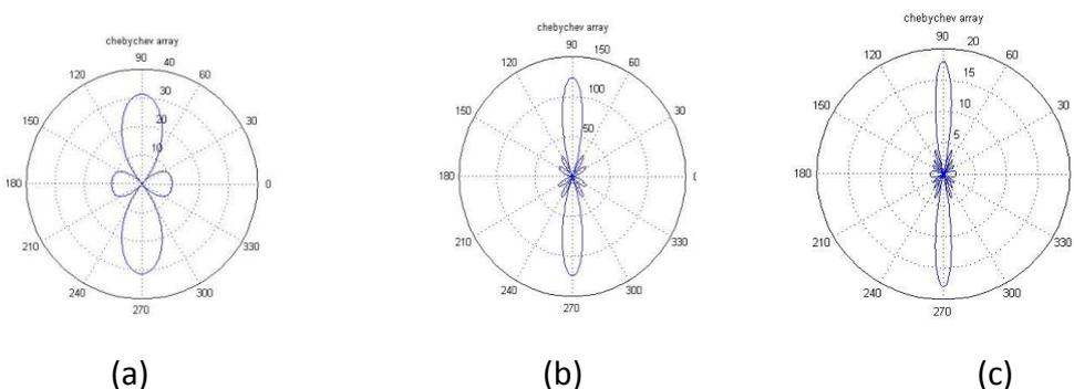
Figure:5 (a)Chebyshev Arrays radiation pattern for n=3, (b) Chebyshev Arrays radiation pattern for n=6, (c) Chebyshev Arrays radiation pattern for n=9
