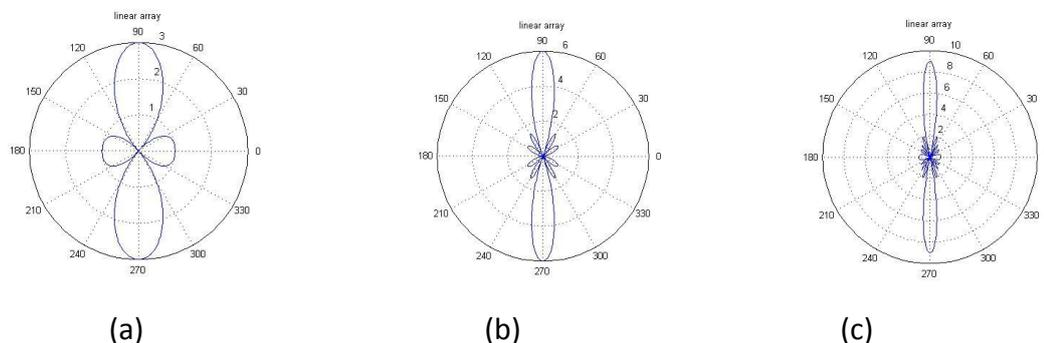
Figure 3.(a) Linear Arrays radiation pattern for n=3, (b) Linear Arrays radiation pattern for n=6, (c) Linear Arrays radiation pattern for n=9
