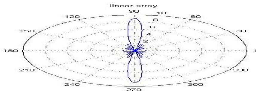
**Figure 2:** Radiation pattern for linear array with n isotropic point sources with equal amplitude and spacing
