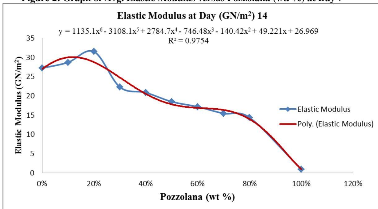
Figure 3: Graph of Avg. Elastic Modulus versus Pozzolana (wt. %) at Day 14
