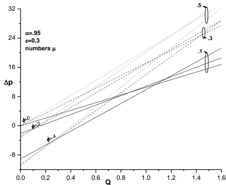
**Fig.4 Pressure drop,  $\Delta p$  versus flow rate,  $Q$  for different  $\mu$  and  $\phi$**
