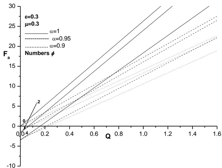
Fig.8 Friction force at tube wall,  $F_a$  versus flow rate,  $Q$  for different  $\alpha$  and  $\phi$ .
