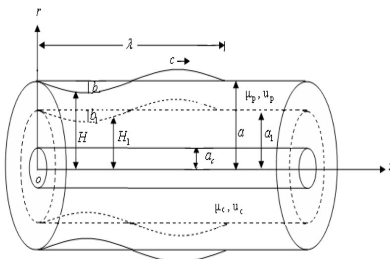
Fig.1 Flow geometry of a two-layered peristaltic pumping in a catheterized tube .
