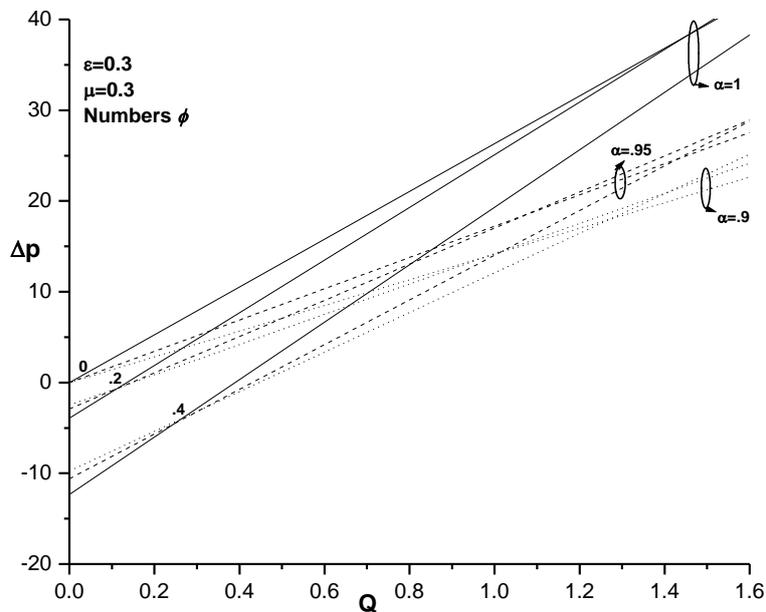
Fig.2 Pressure drop,  $\Delta p$  versus flow rate,  $Q$  for different  $\alpha$  and  $\phi$ .
