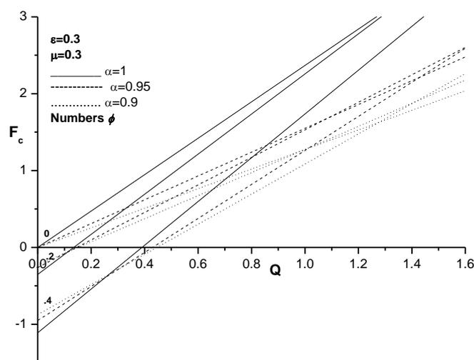
**Fig.10** Friction force at tube wall,  $F_c$  versus flow rate,  $Q$  for different  $\alpha$  and  $\phi$ .
