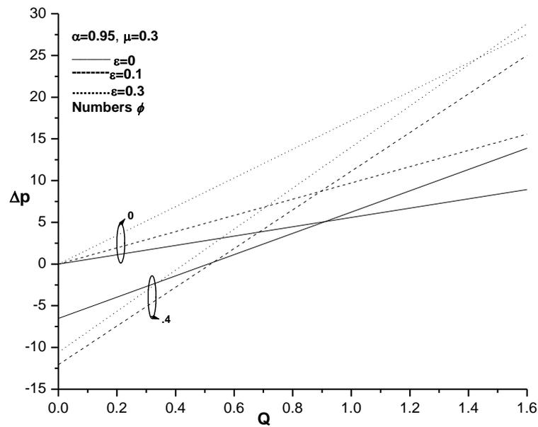
**Fig.5 Pressure drop,  $\Delta p$  versus flow rate,  $Q$  for different  $\varepsilon$  and  $\phi$ .**
