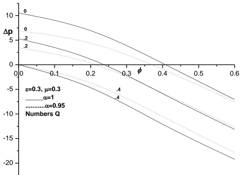
**Fig.6 Pressure drop,  $\Delta p$  versus  $\phi$  for different  $\alpha$  and  $Q$ .**
