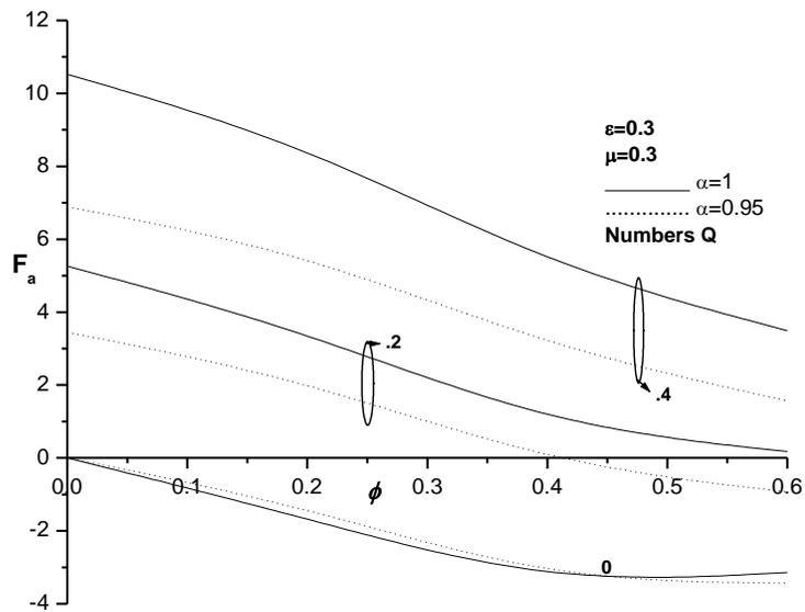
**Fig.9** Friction force at tube wall,  $F_a$  versus flow rate,  $\phi$  for different  $\alpha$  and  $Q$ .
