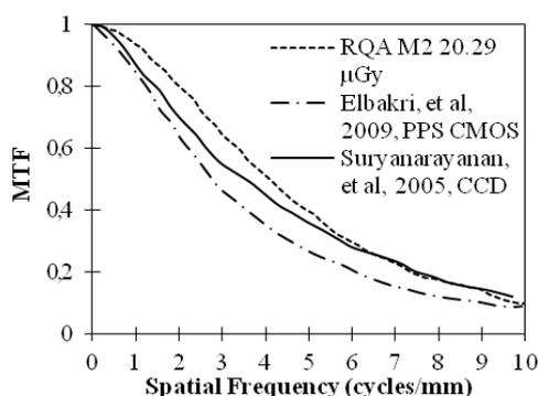
**Fig. 3:** Comparison between the MTF curves of the CMOS detector under investigation, a passive CMOS sensor and a CCD sensor for RQA M2 beam quality.
