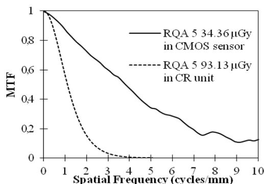
**Fig. 4:** MTF curves for the CMOS sensor (34.36  $\mu\text{Gy}$ ) and the CR unit (93.13  $\mu\text{Gy}$ ) for the RQA 5 beam quality.
