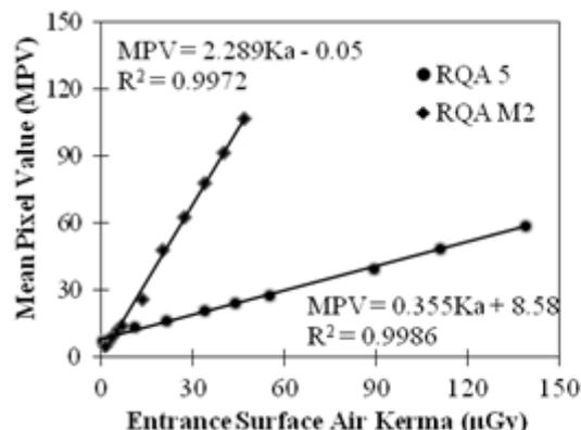
Fig. 1: STP curves for RQA 5 and RQA M2 beam qualities.
