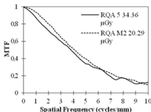
Fig. 2: MTF curves for the RQA M2 (20.29  $\mu\text{Gy}$ ) and RQA 5 (34.36  $\mu\text{Gy}$ ) beam qualities.
