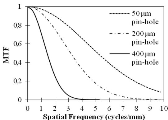
**Fig. 5:** MTF curves by measuring PSF using pin-hole phantoms of 50, 200 and 400  $\mu\text{m}$  diameter respectively method for the RQA 5 (63.65  $\mu\text{Gy}$ ) beam quality.
