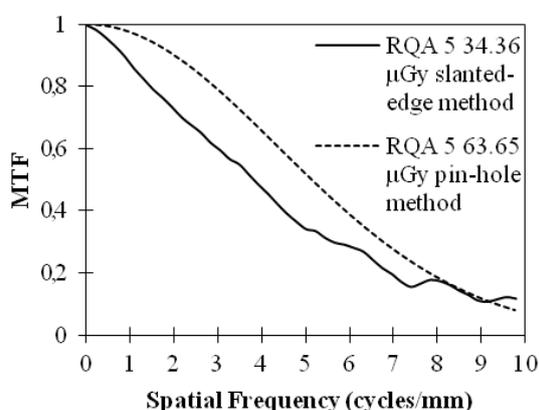
**Fig. 6:** Comparison of the MTF curves of the slanted-edge (34.36  $\mu\text{Gy}$ ) and the pin-hole (63.65  $\mu\text{Gy}$ ) for the RQA 5 beam quality.
