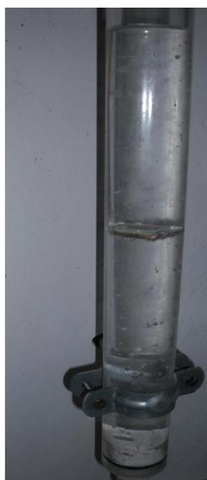
Figure 1. The sedimentation apparatus used for the production of  $\text{Gd}_2\text{O}_2\text{S:Eu}$  phosphor screens.
