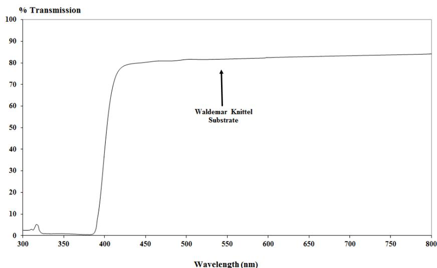
Figure 2. The normalized optical transmission of the rectangular Borosilicate glass substrate 22x22 mm<sup>2</sup> with thickness of 0.13-0.17 mm (Waldemar Knittel-GmbH), using a Perkin-Elmer UV/Visible lambda 15 Spectrophotometer
