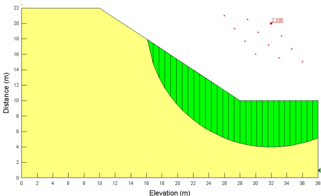
Fig.4 slope type 2 with soil type 1 under OMC condition
