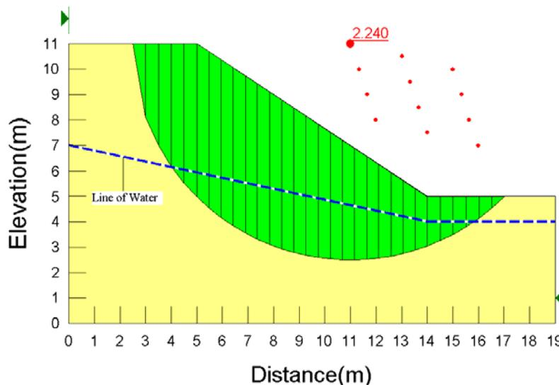
Fig.1 slope type 1 with soil type 1 under saturated condition
