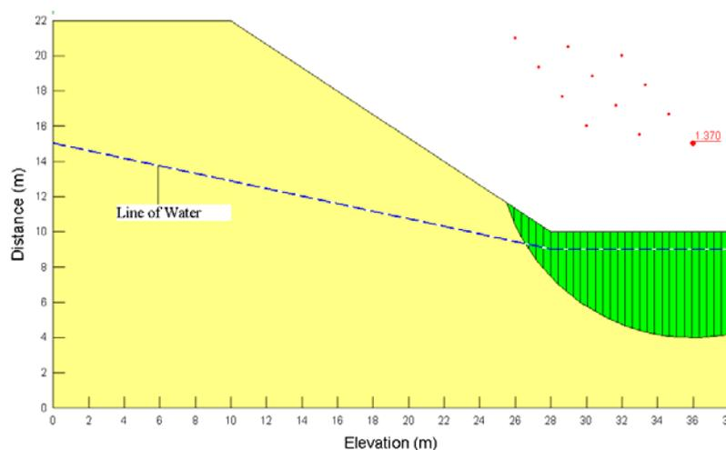
Fig.2 slope type 2 with soil type 1 under saturated condition
