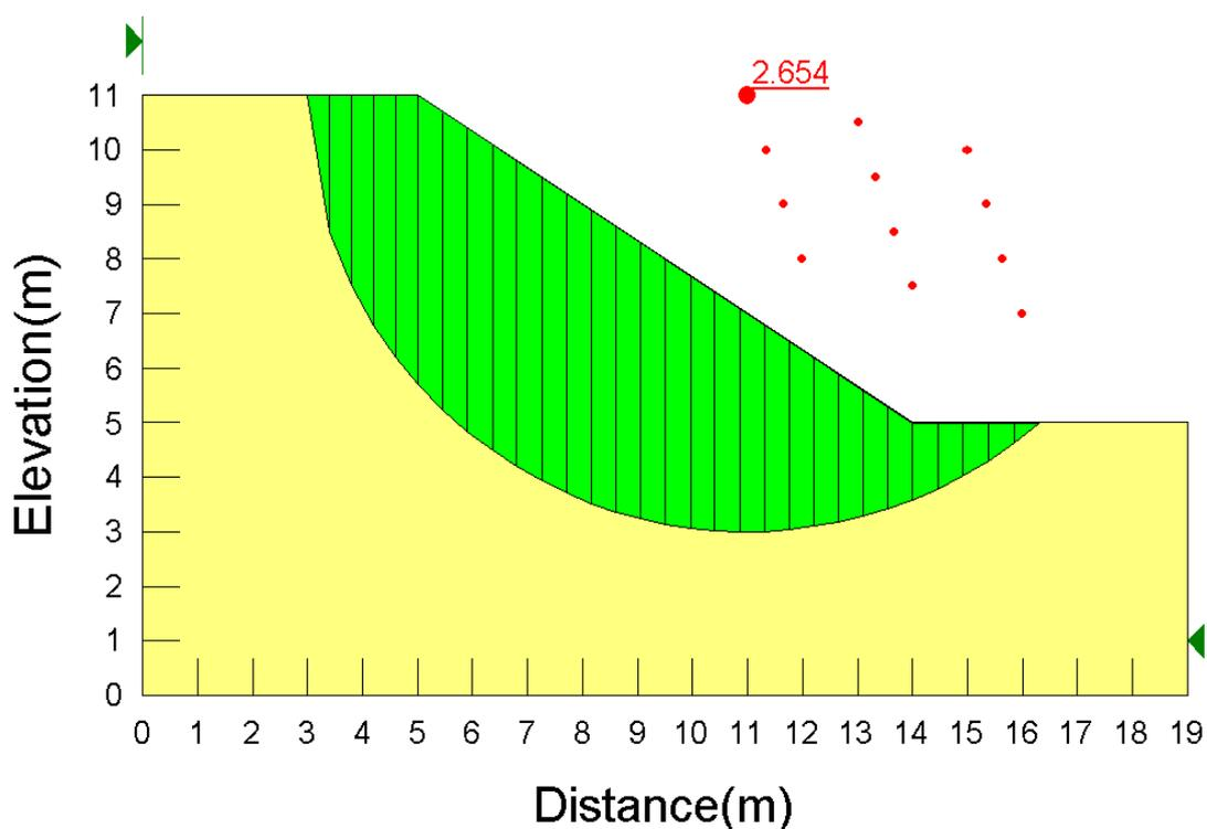
Fig.3 slope type 1 with soil type 1 under OMC condition
