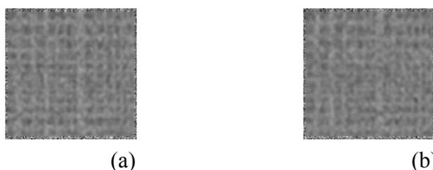
Figure 5. Images taken at the output of the detector for 12cm tissue thickness, 0.08cm microcalcification thickness and 80 and 90kV respectively.
