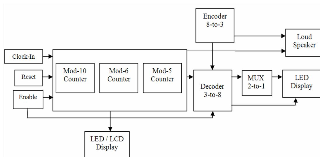
Figure – 2: Basic Hardware of ASIC device
