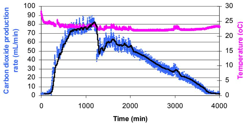
Figure 4. Measurement of the carbon dioxide during fed-batch fermentation of substrate with sugar concentration 100g/L and temperature 22°C. Black line represents the mean value of CO<sub>2</sub> flow per hour.
