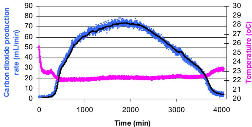
Figure 2. Measurement of the carbon dioxide during the fermentation of substrate with sugar concentration 100g/L and temperature 22°C. Black line represents the mean value of CO<sub>2</sub> flow per hour.
