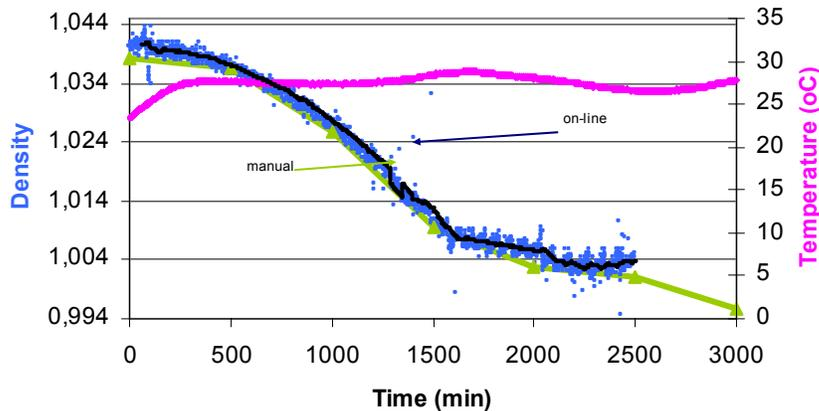
Figure 6. Measurement of the density during fed-batch fermentation of substrate with sugar concentration 100g/L and temperature 30°C, with CO<sub>2</sub> flow meter attached, after system improvement.
