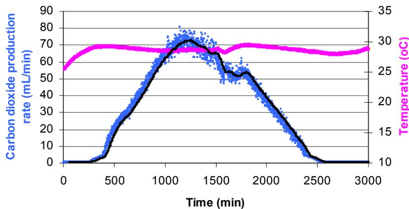
Figure 3. Measurement of the carbon dioxide during the fermentation of substrate with sugar concentration 100g/L and temperature 30°C. Black line represents the mean value of CO<sub>2</sub> flow per hour.
