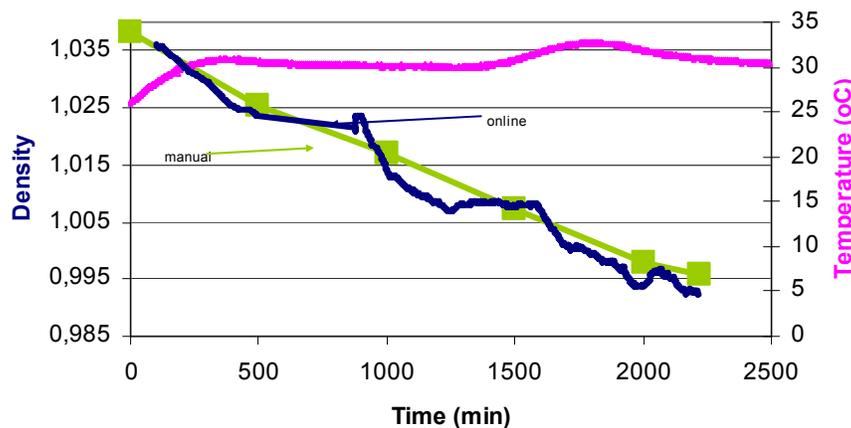
Figure 5. Measurement of the density during fed-batch fermentation of substrate with sugar concentration 100g/L and temperature 30°C, with CO<sub>2</sub> flow meter attached.
