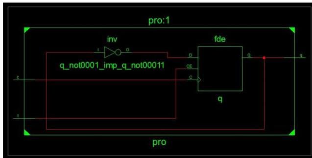
Fig.4.RTL Schematic of LFSR
