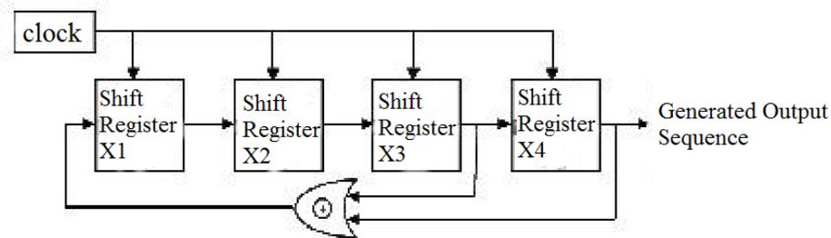
Fig.3. Block Diagram of LFSR
