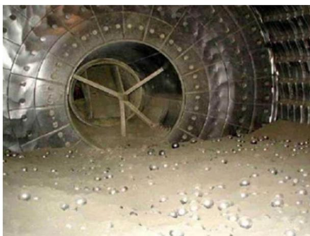
Fig. 1. Internal view of clinker grinding mill
