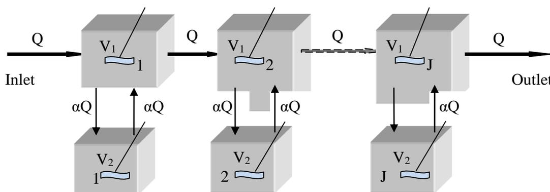
Fig.4: Conceptual representation of perfect mixers-in-series with exchange model.
