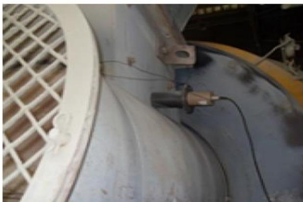
Fig. 2: NaI detector at mill outlet
